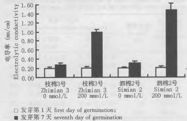
图1 200 mmol/L NaCl胁迫下棉花种子萌发时电导率变化 Fig. 1 Electrolytic conductivities of cotton seeds at first and seventh germination days under 200 mmol/L NaCl stress
