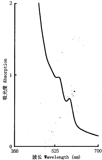
图1 红凤菜红色素水溶液的吸收光谱 Fig. 1 Absorption spectrum of the red pigment solution from Gynura bicolor DC.
